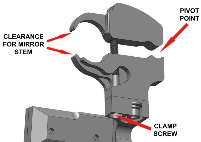
**4 - BEFORE FULLY TIGHTENING THE CLAMP SCREW, POSITION THE MOUNT AS FAR FORWARD TOWARDS THE WINDSHIELD AS YOU CAN. MAKE SURE THE TOP AND MID SECTIONS ARE TOUCHING AT THE PIVOT POINT.** If you can not get them to touch at the pivot point, you have an incompatible mirror type for this mount.
