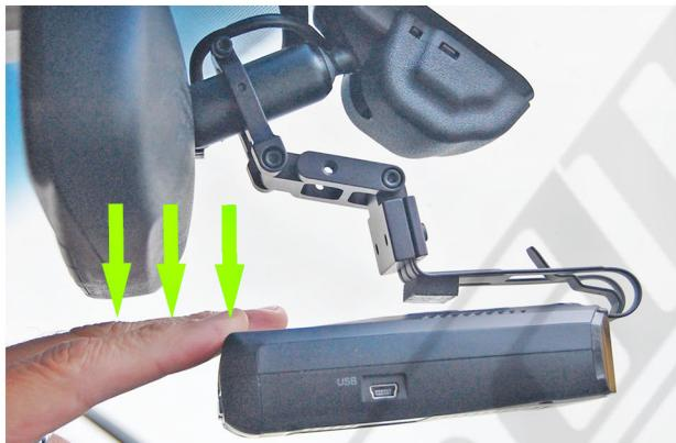
**7 -** If the RD is too close to the bottom of the mirror, You may access the buttons on top of the RD by gently pushing downward on the front of the RD with one finger and push the desired button with another finger. Then allow the RD to return to its original position by gently letting it spring upward. When accessing the buttons, be sure to push the RD downward just enough for your finger to fit between the RD and mirror. **Do not push down more than what is needed.**
