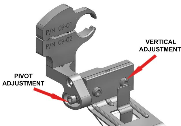
**5 -** When the mount is positioned as far forward as it will go, tighten the clamp screw until the Top and Mid Sections are **slightly snug** around the mirror stem. You should still be able to rotate the mount. Rotate the mount so it is parallel with the bottom of the mirror. Tighten the clamp screw until the mount is securely attached to the mirror stem.
